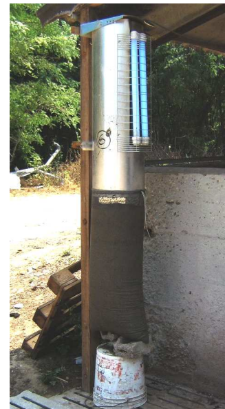
fig. 6: Turbine trap at the maximum capacity. The bag contained more than 16 Kg of mosquitoes collected in a week.
